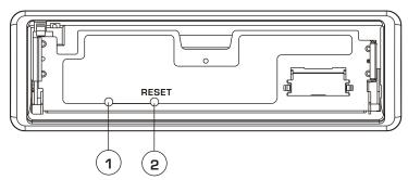
1.LED INDICATOR: Flashing when detachable panel is removed.
